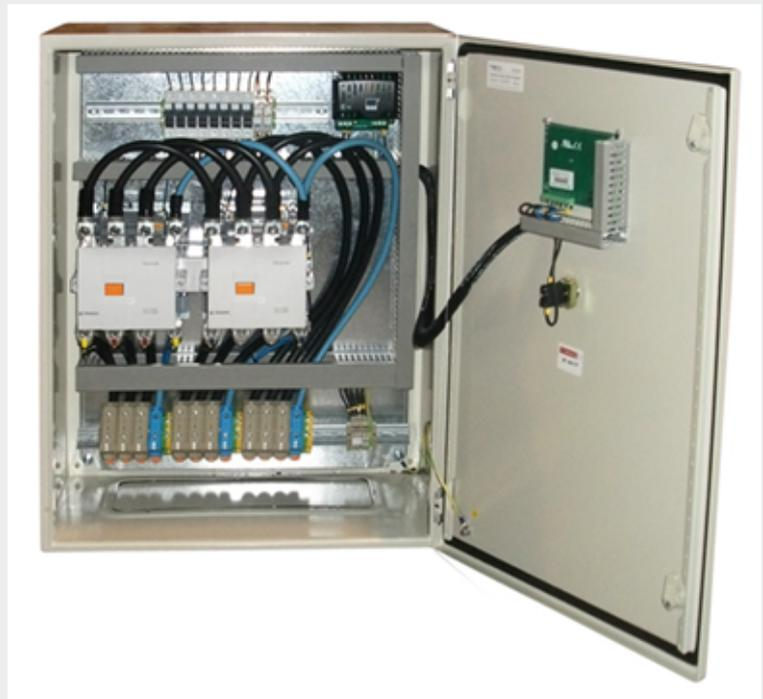
Cubicle composed of the electronic control module which is detecting a mains failure and of 2 contactors mechanically and electrically interlocked or a motorized switch controlled by the above electronic controller who are realizing the change of supply from the GEN SET or the MAINS to the load.
